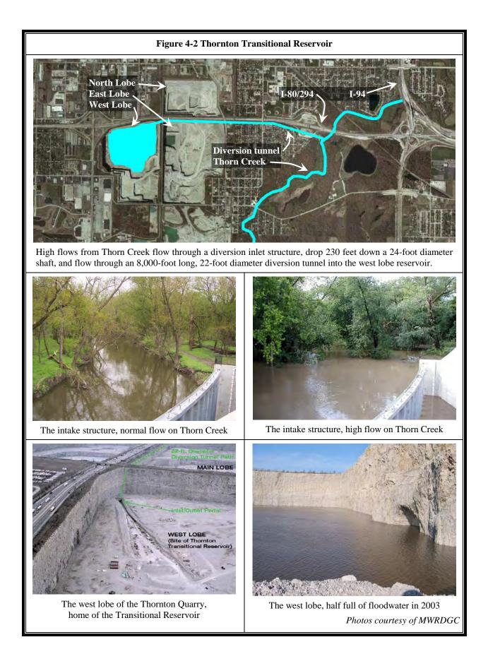
The Thornton Transitional Reservoir provides overbank flood relief for 9 communities and has captured 36 BG of flood water during 56 fill events. The Corps of Engineers estimated that the Thornton Transitional Reservoir would reduce \$135,000 average annual damage to \$300.
