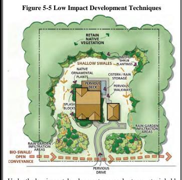
Under the low impact development approach, stormwater is held on the site where it falls. It is allowed to soak into the ground in order to replicate the natural conditions that produce continuing flowing streams with better quality water.
