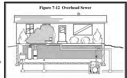
is a permanent alteration to the plumbing. The only concern is when power is lost, the ejector pump won't work. This only limits the use of the facilities in the basement that need the pump. Upstairs plumbing still works.
