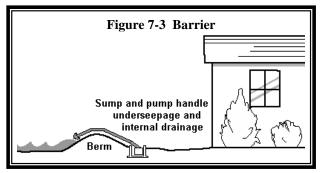
By keeping water away from the building walls, the problems of seepage and hydrostatic pressure are reduced. Basements and the lower floors of split levels can also be protected by construction of low walls around stairwells.
