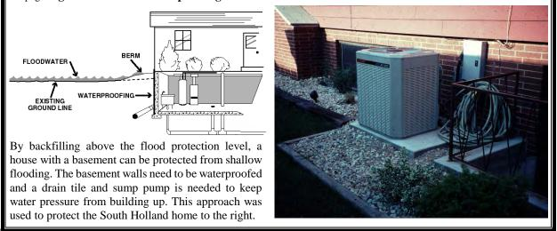
The secret is to not let surface water touch the house. This will greatly increase the amount of water against the basement walls, resulting in much greater hydrostatic pressure. Sump pumps cannot keep up with surface water. An example of this backfill or waterproofing berm approach is in Figure 7-6.
